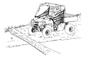
5. Always have all passengers dismount and move away from the vehicle before operating over an obstacle that could cause a rollover.
